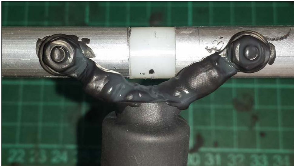
Photo 1: An open feed-point example, the feed should be as close to a 'T' shape as possible
